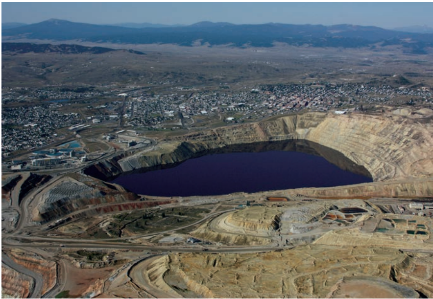
The Berkeley Pit is a former open pit copper mine located in Butte, Montana. It is one mile long by half a mile wide with an approximate depth of 1,780 feet (540 m). It is filled to a depth of about 900 feet (270 m) with water that is heavily acidic (2.5 pH level). As a result, the pit is laden with heavy metals and dangerous chemicals that leach from the rock, including arsenic, cadmium, zinc and sulfuric acid. http://en.wikipedia.org/wiki/Berkeley_Pit
