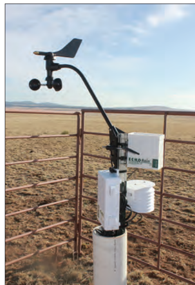
Figure 3. A Decagon™ micro-climate and hydrology monitoring station at Piojo Ranch provides instant information on weather and soil conditions.
