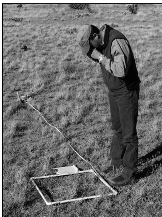
Photo 24: Photo of "Quadrat" along tape measure. The quadrat's lower left-hand corner is placed at the 3-meter mark on the opposite side of the tape of the photographer. The photographer should stand so that the feet are nearly touching the tape measure. This will ensure that the photo is taken looking straight down on the quadrat. Place the notebook in the scene to help identify the photo.
