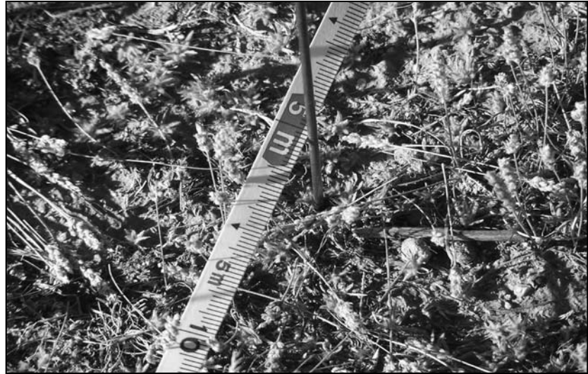
Photo 25: Left photo of lowering the steel rod to the soil surface. Photo 26: Above, photo shows a close up of the contact between the point of the rod and litter cover at the 5 meter mark on the tape.
