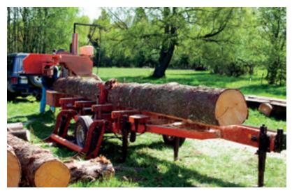
An example of a portable sawmill. Micrologging is handy for thinning overgrown forests, has low labor costs, and can provide a convenient source of wood. *Photo by bright/Shutterstock*
