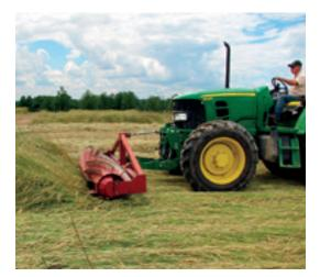
The roller-crimper in action (Jeff Moyer on tractor). A cover crop is crimped in the spring to smother weeds and protect the cash crop. *Photo courtesy of the Rodale Institute*
