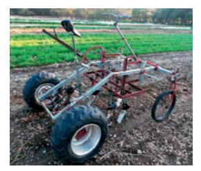
An example of Farm Hack innovation: the "culticycle" is a pedal-powered tractor for cultivation and seeding, built from lawn tractor, ATV, and bicycle parts. *Photo courtesy of Dorn Cox*
