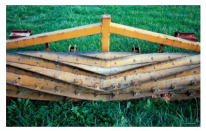
Detail of a roller-crimper, the key piece of equipment in an organic no-till farming system. *Photo by Courtney White*
