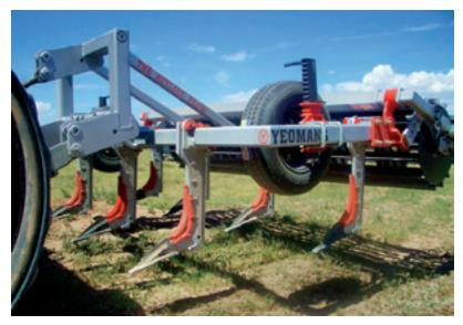
A Yeomans Plow "rips" a 10-inch-deep furrow in compacted soil, allowing water to feed soil microbes, thus building topsoil. *Photo courtesy of Owen Hablutzel*
