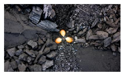
Eight different biochars made from various types of wood and nut shells, with corn seeds for scale. *Photo courtesy of Josiah Hunt*
